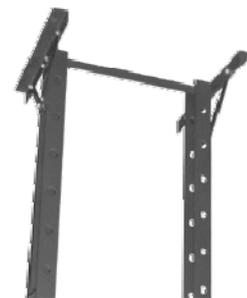
Attach return springs 14 to the cross beam 1. Locate Jack plate 3 and position parallel to cross beam.
