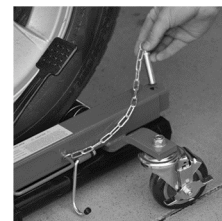
8. Install safety locking pin and put castor lock in "on" position then repeat steps 1-8 on opposite wheel/s.
