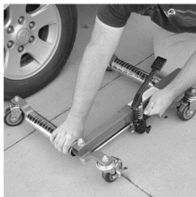
5. Spread jack arms apart until they fit the vehicle wheel. You must leave 20mm gap between tyre and jack.
