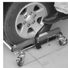
7. Pump foot pedal until vehicle is raised from the ground and the locking pin hole is exposed.
