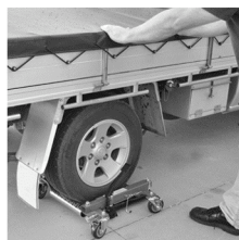
9. Once the vehicle is raised on both sides or all four wheels and the castor locks all turned off, it can easily be moved by pushing on the side of the vehicle to the desired position.
