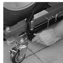
11. To lower vehicle put castor lock into "off" position, remove safety locking pin, and open pump valve.
