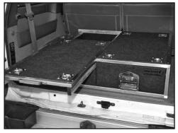
Remove right hand side top section by undoing the 10 retaining screws and set aside taking care not to loose the fasteners and remove/open the fridge slide by sliding outwards. This allows access to the internal base of the drawer system so it can be bolted to the vehicle
