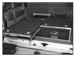
Once the mounting bolts are secure refit or close the fridge slide, re attach the right-hand top section and trim ensuring all fasteners are tightened.
