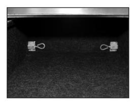
Remove the 2 drawers by unlatching the 2 retaining latches located at the rear interior of the drawer
