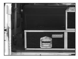
Once the mounting bolts are secure,re attach the top section and trim ensuring all fasteners are tightened.
