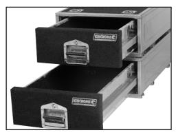
To stack a second drawer system on top of another fitted unit remove the drawer and line up the base mounting slots with lower unit mounting holes on the lower unit. Install the stacking bolts and ensure they are tight.
