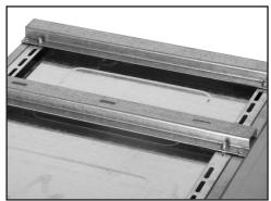
Check the base of the vehicle that the drawer system is to be installed in and identify suitable mounting points within the vehicle. Either use existing vehicle mounting points or new drill new mount points using the bottom fixing ribs as a guide for drilling the holes or locating to existing mounting points.
