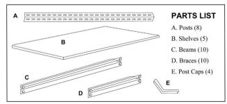
Assembly is done by fitting the rivets of the beams and braces into the post slots.
