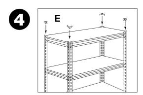
Add a shelf to the previously built level, then continue by adding the fourth and fifth level to the unit using two beams and two braces per level. Tap lightly to properly seat the rivets and add the final shelves to the unit. Install all four end caps to the top of the unit after assembly has been completed (**E**). Install end caps to post by pressing down on ends.
