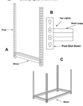
Start by adding a shelf to the level previously built, then continue working by adding the second level using two (2) beams and two (2) braces in the post slots of your desired location.
