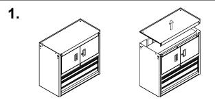
REMOVE UNIT FROM CARTON AND STAND UNIT UPRIGHT. REMOVE CABINET TOP BY LIFTING STRAIGHT UPWARD AND SET ASIDE.
