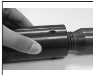
Fasten Needle Scaler to Air Hammer.
