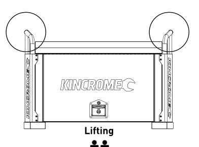
Use roll cage carry points to lift. NOTE: Manual lift only when empty. Mechanical assistance is recommended.
