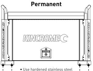
bolts & fasteners with appropriate thread locker or locking nuts when mounting to vehicle trays.
