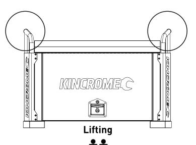
Use roll cage carry points to lift. **NOTE:** Manual lift only when empty.
